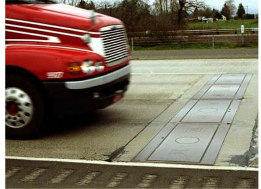
*Scales in the pavement weigh trucks as they pass while sensors above check their credentials.*
