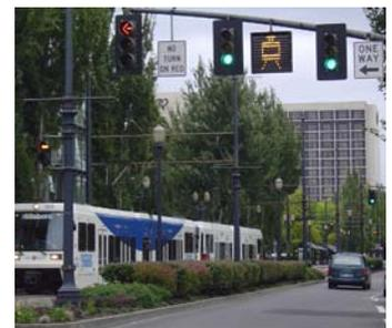
*Signal technology at this intersection keeps cars from turning when a train is approaching.*
