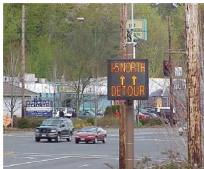
*When Barbur Boulevard is used as a detour for traffic stuck on I-5, variable message signs can help direct traffic back to I-5 at the appropriate time.*
