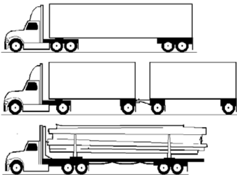
Tractor (TR) - a motor vehicle designed and used exclusively to pull trailers.
