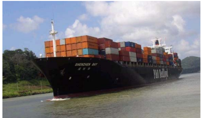
Panamax ship carrying containers through Panama Canal, courtesy Wikipedia. The Free Encyclopedia
