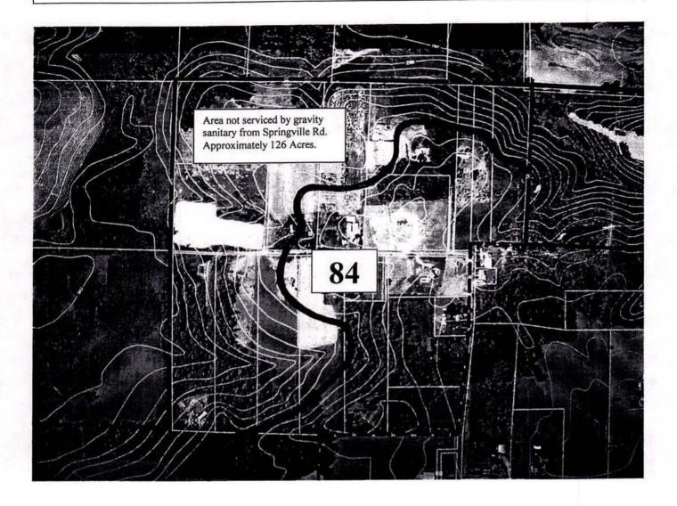
The red line on this exhibit indicates the approximate limits of gravity sewer service available in area 84 due to topography constraints.
