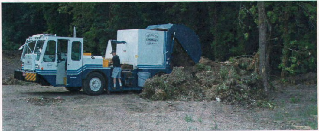
Wacker.04AUG09.dka.p04 Compactor truck tipping yard debris.
