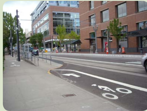
This bike lane in Portland leads cyclists safely behind a streetcar stop, out of the way of both vehicles and waiting pedestrians.
