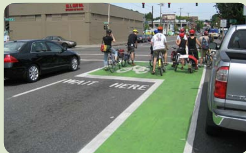
A bike box in Portland allows cyclists to be more visible at intersections.
