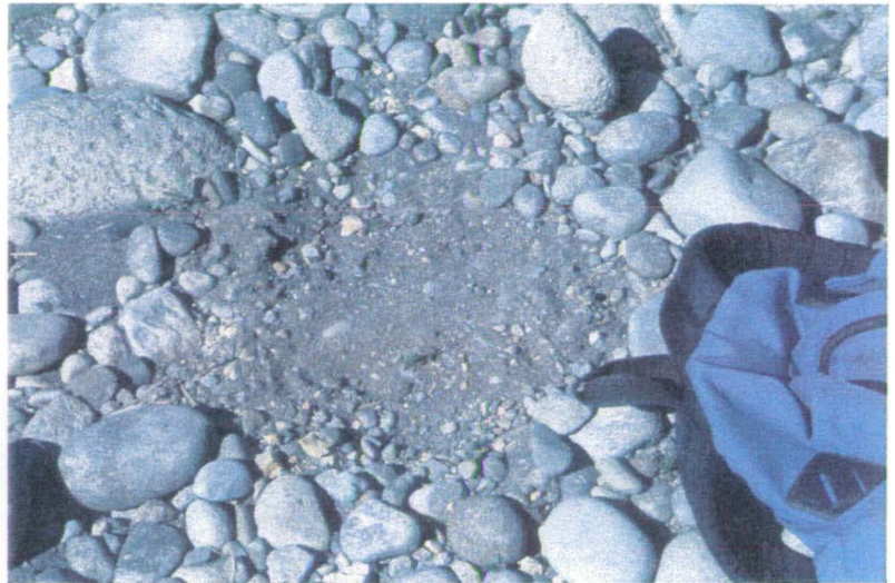
Left: Measuring sediment grain size along a cross-channel transect. Above: Fine sediments beneath the armoring layer on the bar at the launching area. Below: "Skeletal" point bar at the launch area, with eroding bank directly upstream.
