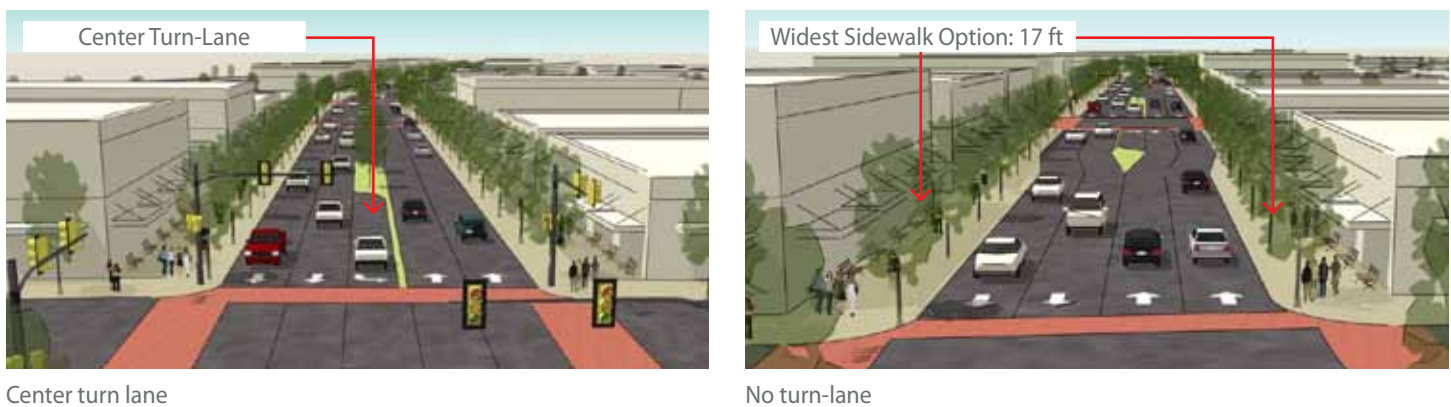
FIGURE 13: CROSS SECTIONS OF PROPOSED CANYON ROAD INTERSECTIONS
