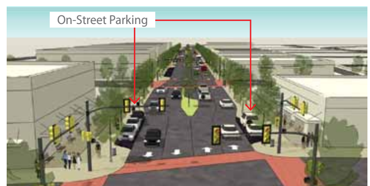
On-street parking, both sides. This design is only applicable for limited areas due to sidewalk width needs.
