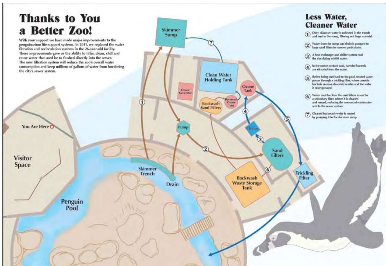
The updated filtration system in the penguin exhibit at the Oregon Zoo reduces water usage by 90 percent in the exhibit.
