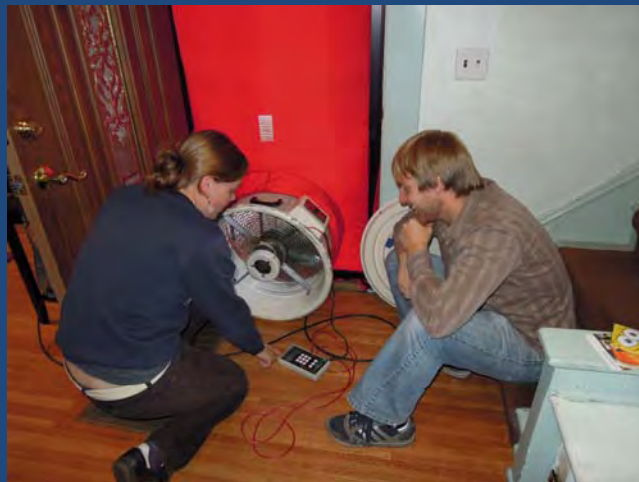
Hands-on Blower Door Testing training with AmeriCorps CEC member and OIT Intern
