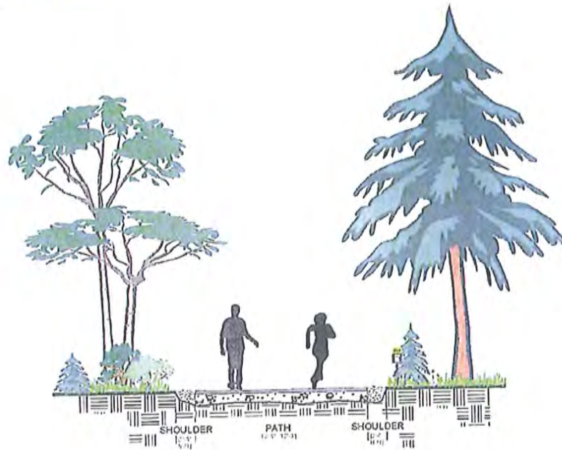
Figure 1 – Typical cross-section for a shared use path
