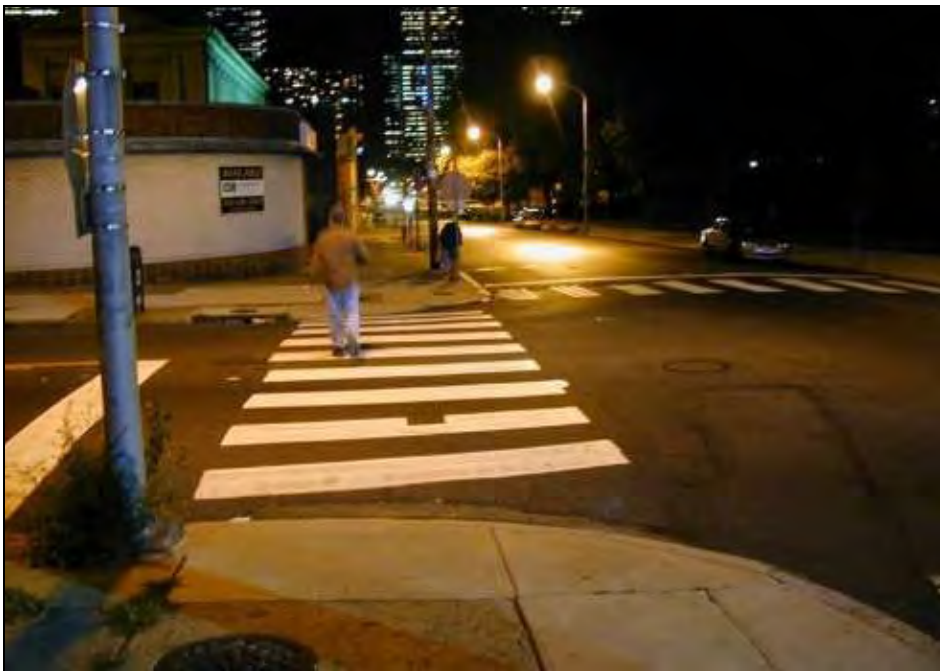
Lighting is a crucial part of pedestrian and bicycle safety. Lighting intersections and routes makes it easier for pedestrians and bicyclists to be seen. Photo: Michael Ronkin.
