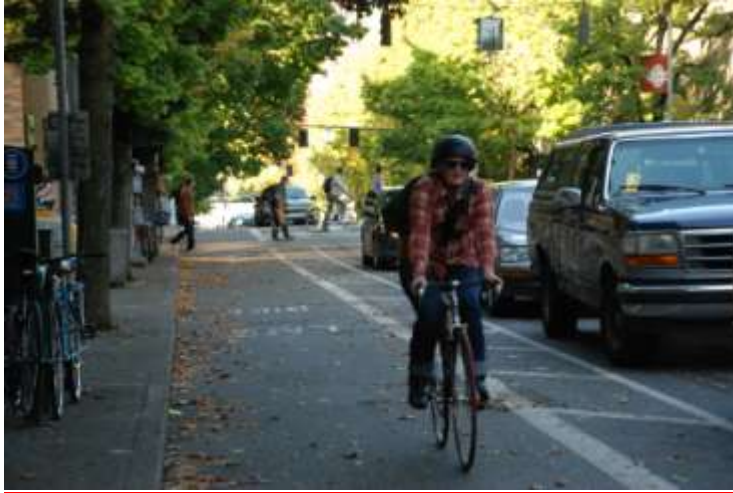
Providing separation for people walking and riding bicycles can make the road safer and easier to navigate for all users. Moving parked cars over provides a cycle track near Portland State University. Photo: City of Portland
