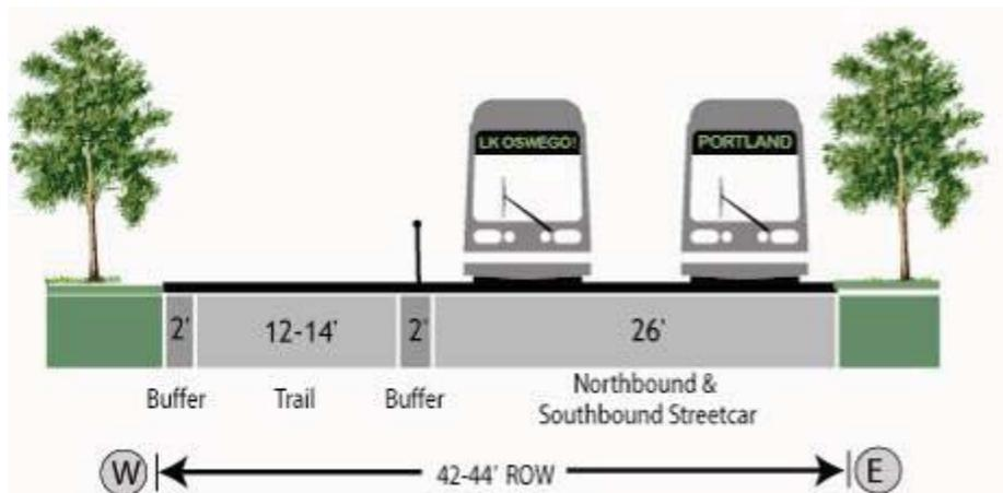
**Figure 41. Section 1.9a Willamette Shore Line with Double-track Streetcar**
