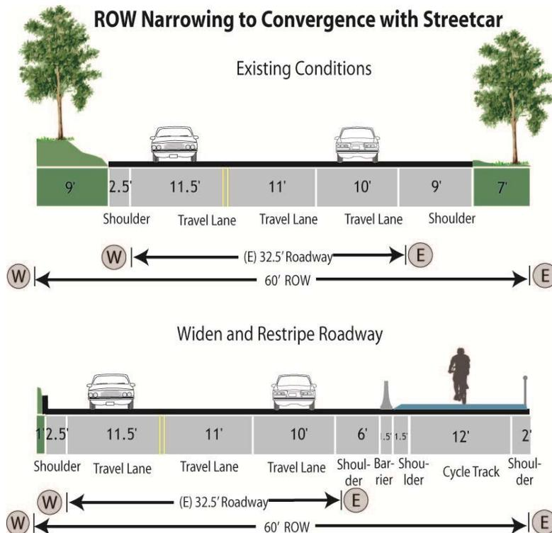
Figure 70. Conceptual Section 3.1b7- Widen Trail 7' (E), Widen Roadway 8' (W), Restripe for 244'
