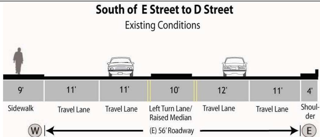
**Figure 78. Conceptual Section 3.2c5 - BIKE LANES CANNOT BE ACCOMODATED for 210'**
