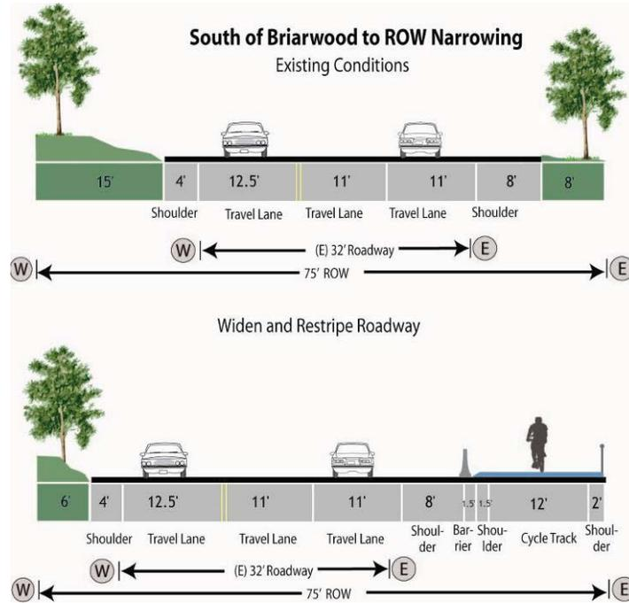
Figure 69. Conceptual Section 3.1b6- Widen Trail 8' (E), Widen Roadway 9' (W) and Restripe 220'
