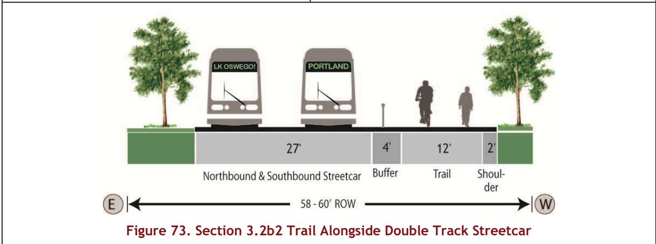
**Figure 73. Section 3.2b2 Trail Alongside Double Track Streetcar**
