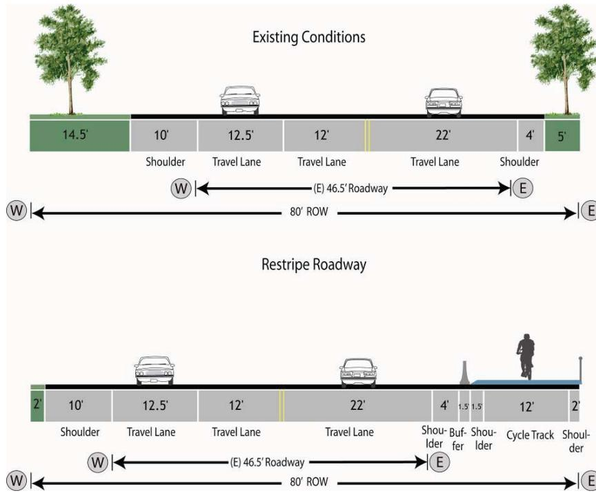
Figure 49. Conceptual Section 2.3.2- Widen Trail 5' (E), Widen Roadway 12.5' (W), Restripe 275'
