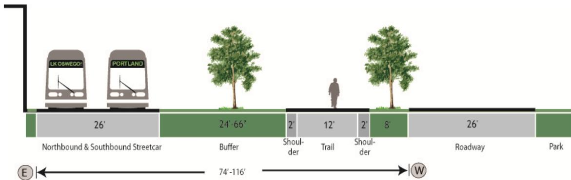
**Figure 33. Section 1.5a1 Willamette Shore Line with Double-track Streetcar**
