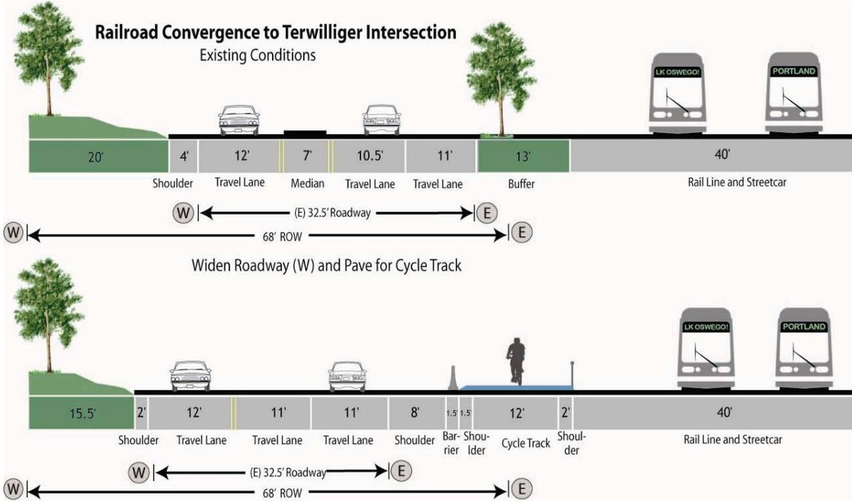
**Figure 75. Conceptual Section 3.2c2 - Cycle Track between Roadway and Streetcar/ Railroad 256'**
