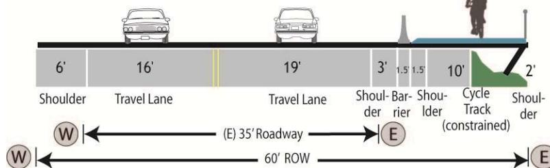
Figure 59. Conceptual Section 2.4b3- Widen Bench Cycle Track onto Roadway, Restripe for 525'
