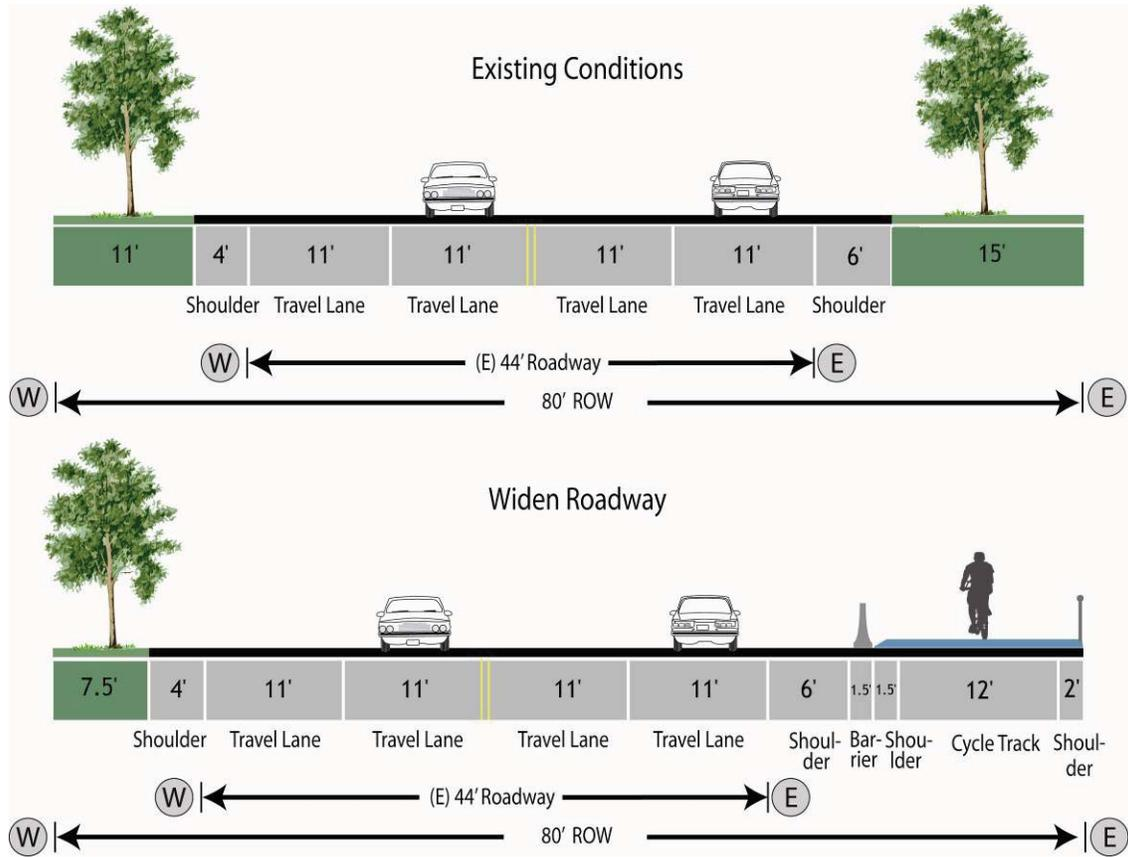
**Figure 48. Conceptual Section 2.3.1 - Widen Trail 15' (E), Widen Roadway 3.5' (W), Restripe for 130'**
