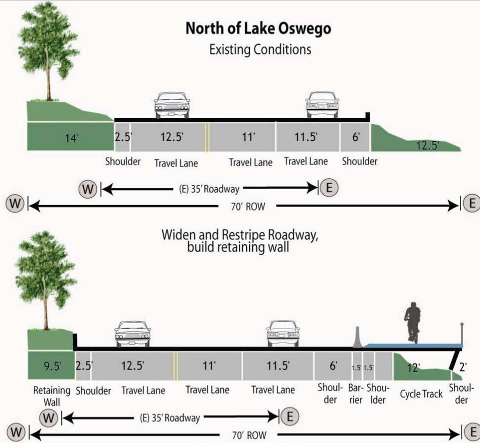
**Figure 62. Conceptual Section 2.4b6- Widen Roadway 5' (W), add Retaining Wall, Bench Cycle Track onto Roadway and Restripe for 596'**
