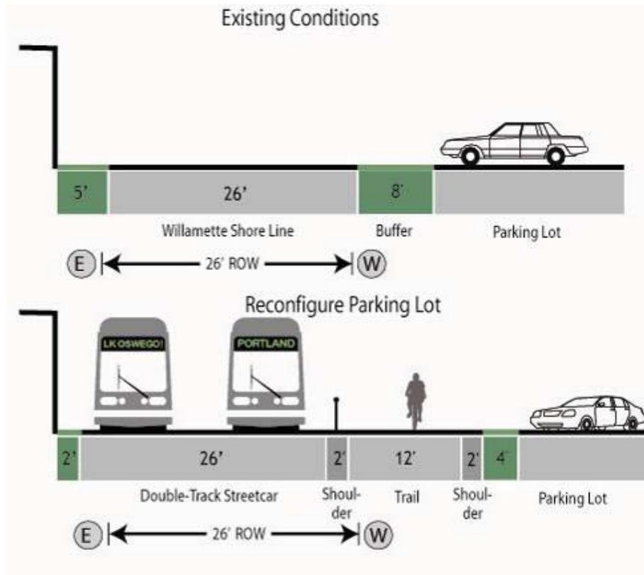
**Figure 25. Section 1.1a Willamette Shore Line with Double-track Streetcar**
