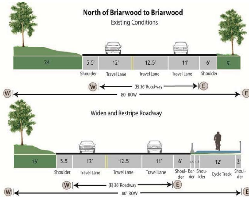
Figure 65. Conceptual Section 3.1b2- Widen Roadway 6' (W), Widen Trail 11' (E), Restripe 792'
