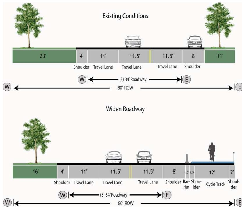
Figure 50. Conceptual Section 2.3.3 - Widen Trail 11'(E), Widen Roadway 7'(W), Restripe 700'
