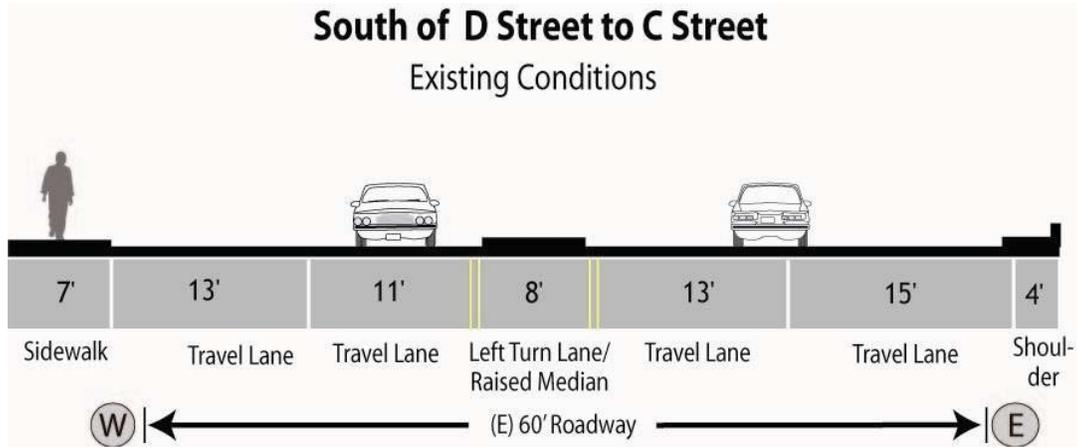
**Figure 79. Conceptual Section 3.2c6 - BIKE LANES CANNOT BE ACCOMODATED for 543'**
