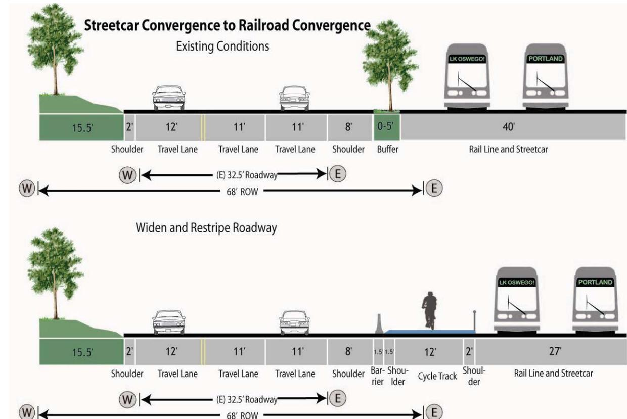
**Figure 74. Conceptual Section 3.2c1- Cycle Track between Roadway and Streetcar for 600'**
