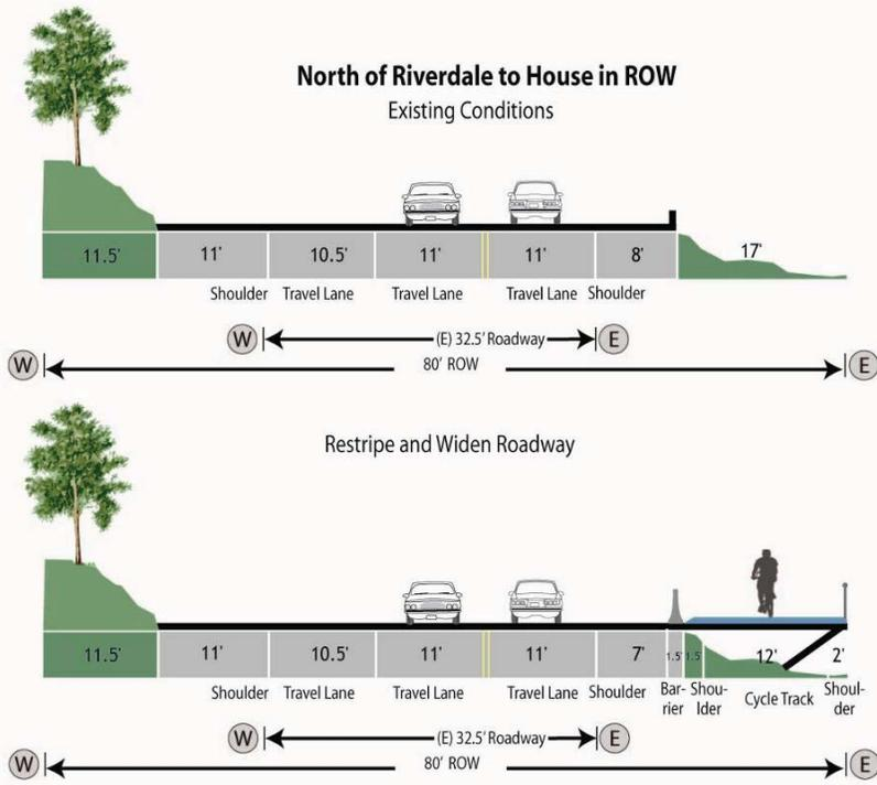
Figure 51. Conceptual Section 2.3.4- Bench Trail onto Roadway for 240'
