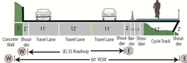
Figure 58. Conceptual Section 2.4b2 - Widen Roadway 5' (W), Bench Cycle Track onto Roadway, Move Concrete Wall, Restripe for 2,324'
