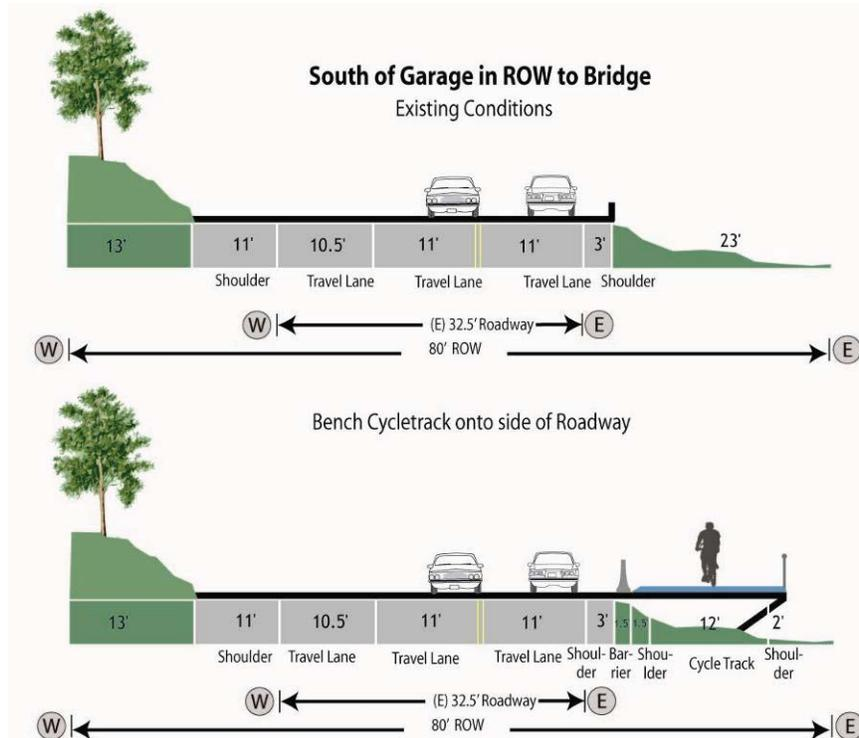
Figure 53. Conceptual Section 2.3.6 - Bench Trail onto Roadway 603'
