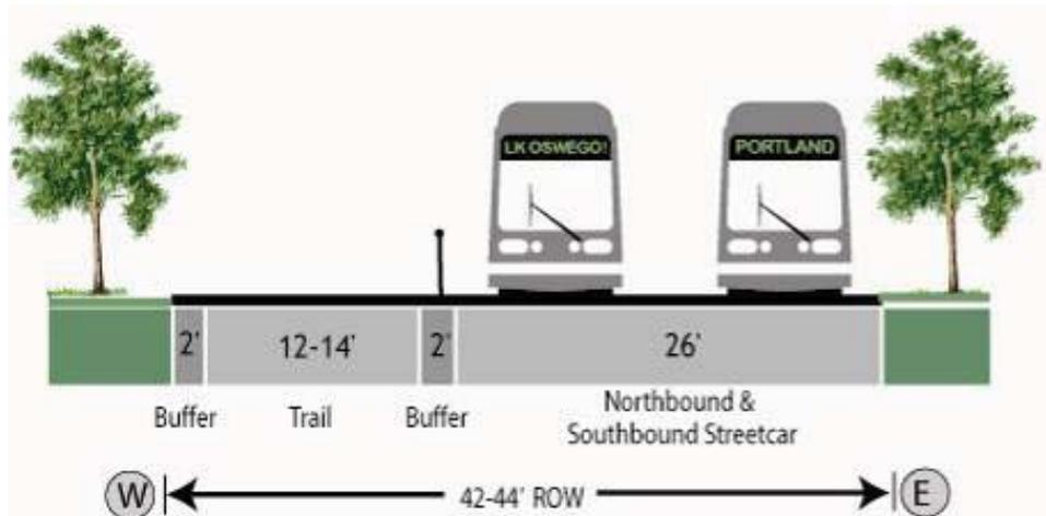
**Figure 39. Section 1.8a Willamette Shore Line with Double-track Streetcar**
