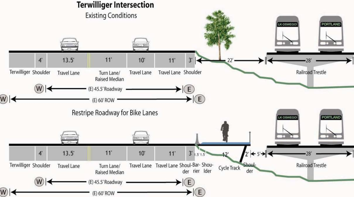
**Figure 76. Conceptual Section 3.2c3 - Cycle Track between Roadway and Streetcar/ Railroad 114'**
