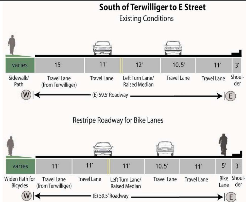
**Figure 77. Conceptual Section 3.2c4 - Narrow Lanes and Restripe Roadway for Bikelanes for 326'**
