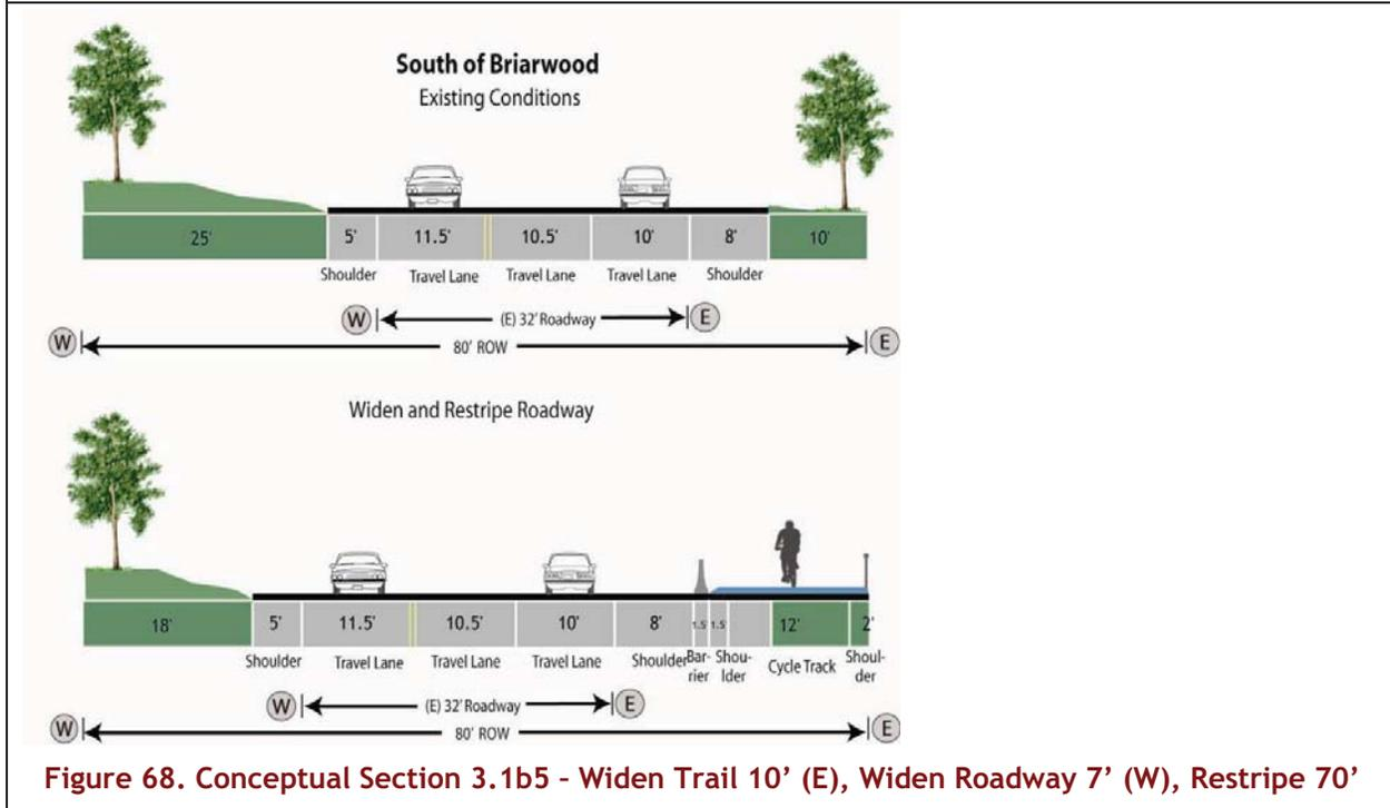
Figure 68. Conceptual Section 3.1b5 - Widen Trail 10' (E), Widen Roadway 7' (W), Restripe 70'
