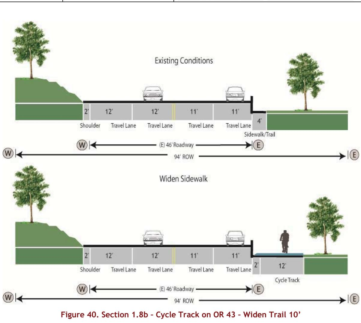
**Figure 40. Section 1.8b - Cycle Track on OR 43 - Widen Trail 10'**
