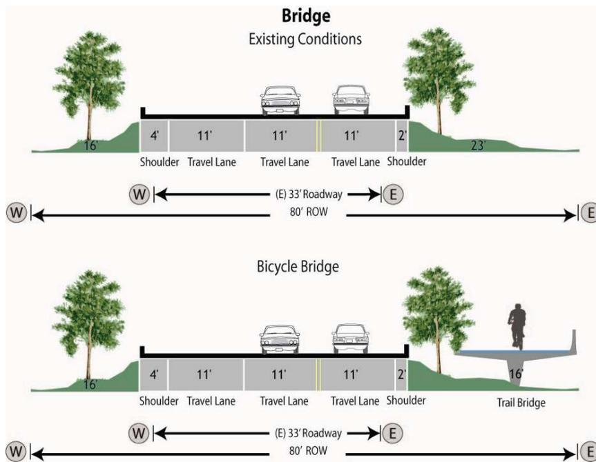
Figure 54. Conceptual Section 2.3.7 - Trail Bridge for 529'
