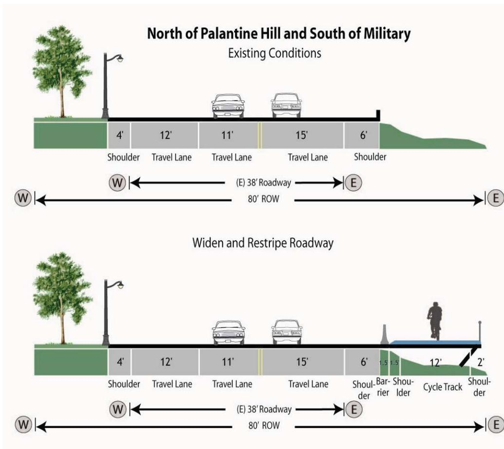
**Figure 57. Conceptual Section 2.4b1 - Bench Trail onto Roadway for 414'**
