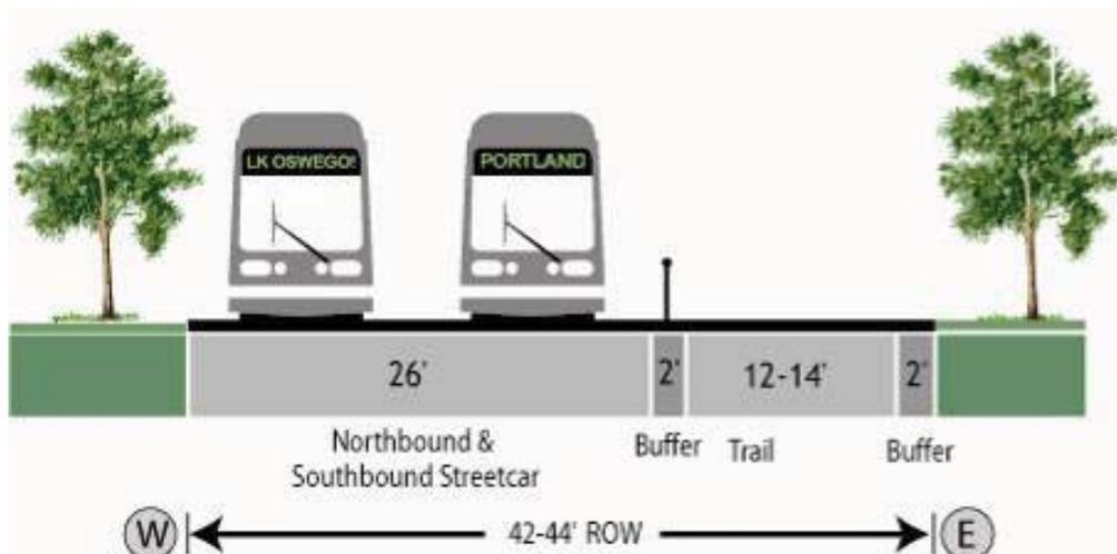
**Figure 56. Conceptual Section 2.4a2 Trail Adjacent to Double-Track Streetcar in Willamette Shore Line**
