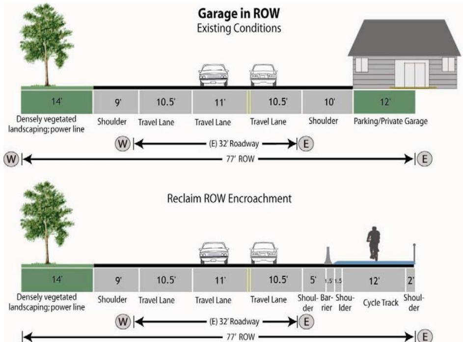
Figure 52. Conceptual Section 2.3.5 - Reclaim Encroachment for 56'
