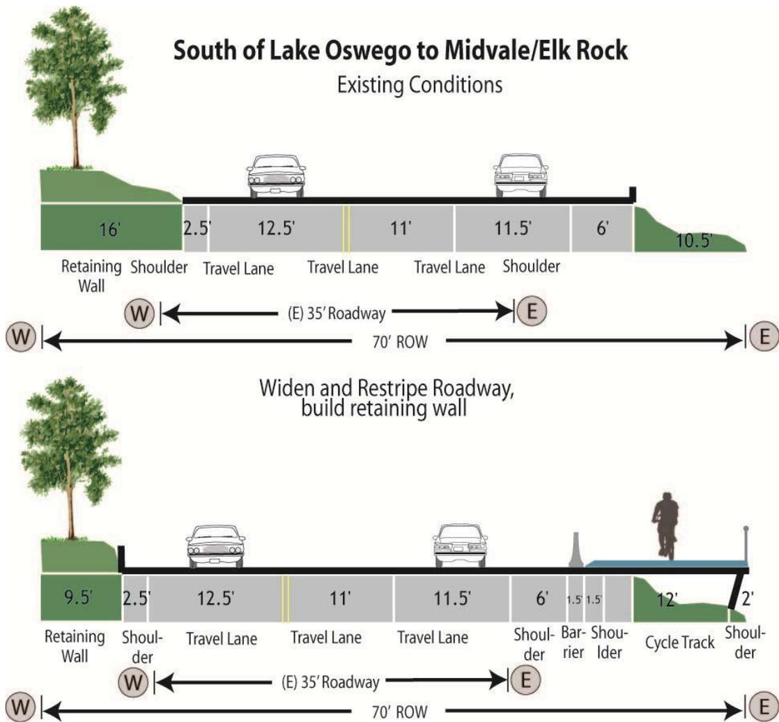
**Figure 64. Conceptual Section 3.1b1- Widen Roadway 6.5' (W), Add Retaining Wall, Bench Cycle Track onto Roadway and Restripe for 518'**
