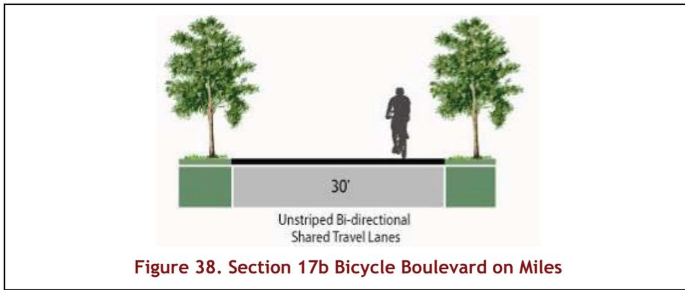
**Figure 38. Section 17b Bicycle Boulevard on Miles**
