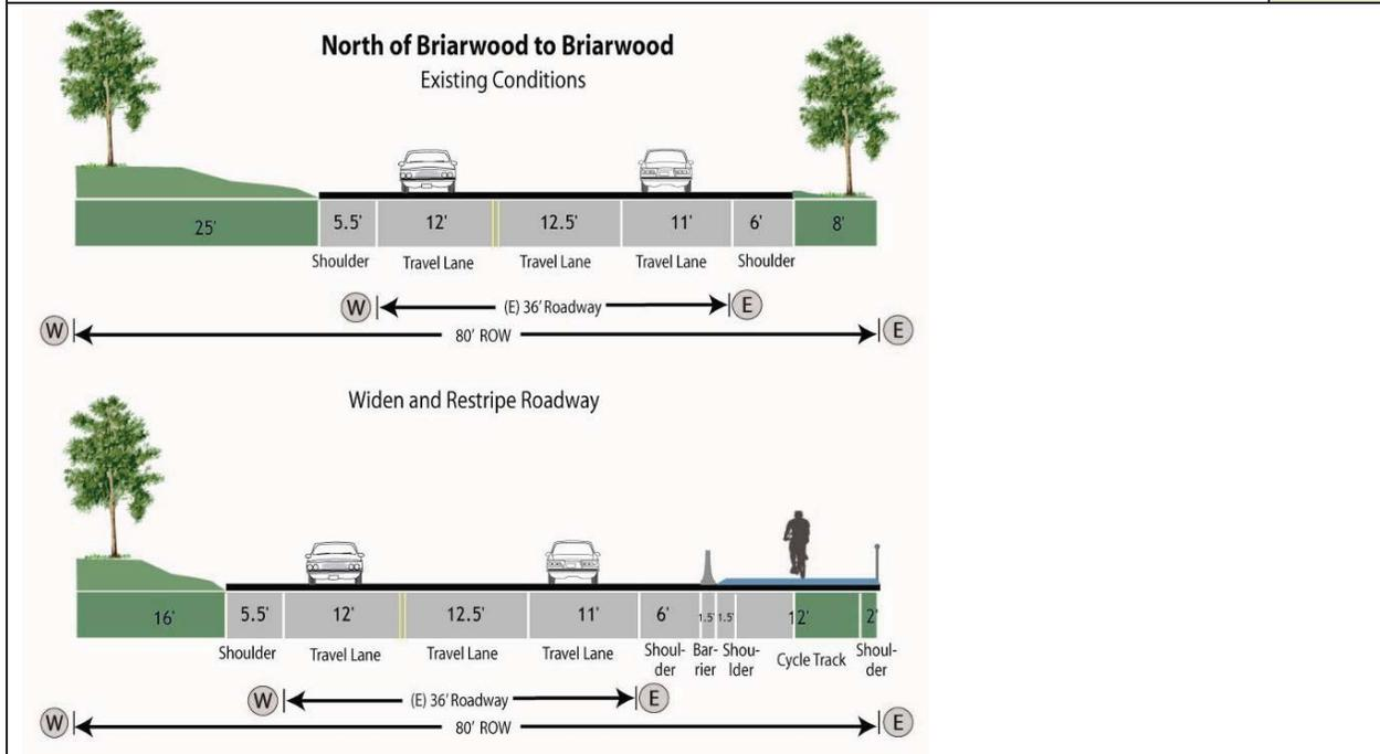
Figure 67. Conceptual Section 3.1b4- Widen Trail 8' (E), Widen Roadway 9' (W), Restripe for 195'
