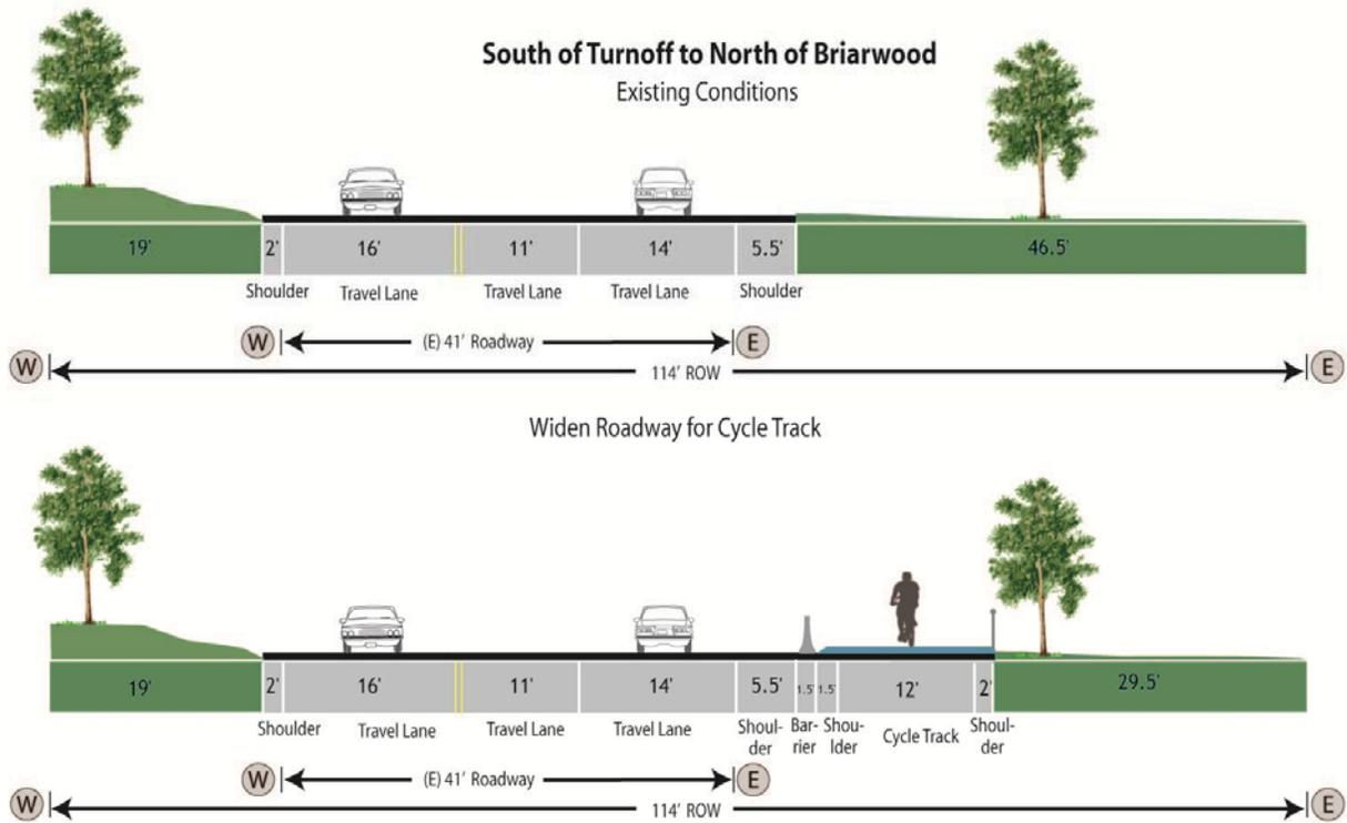
Figure 66. Conceptual Section 3.1b3 - Widen Trail 17' (E) for 198'
