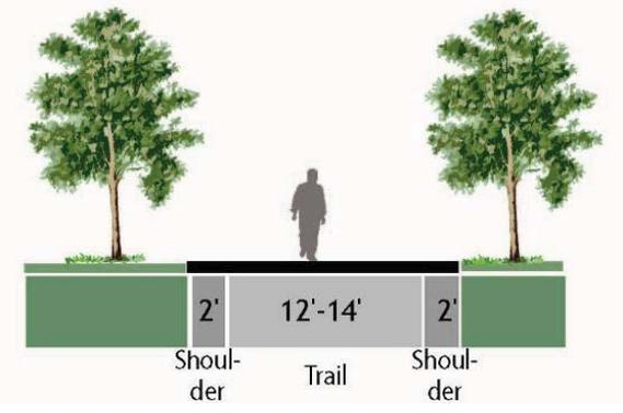
**Figure 27. Section 1.2a Trail Only in Willamette Shore Line**
