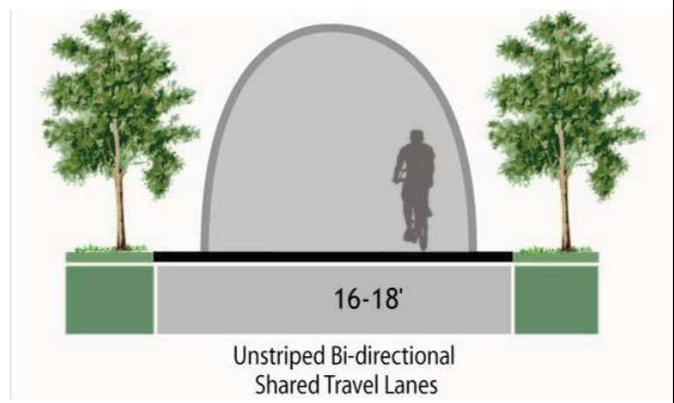
**Figure 71. Section 3.2a Bicycle Boulevard Improvements on Fielding**
