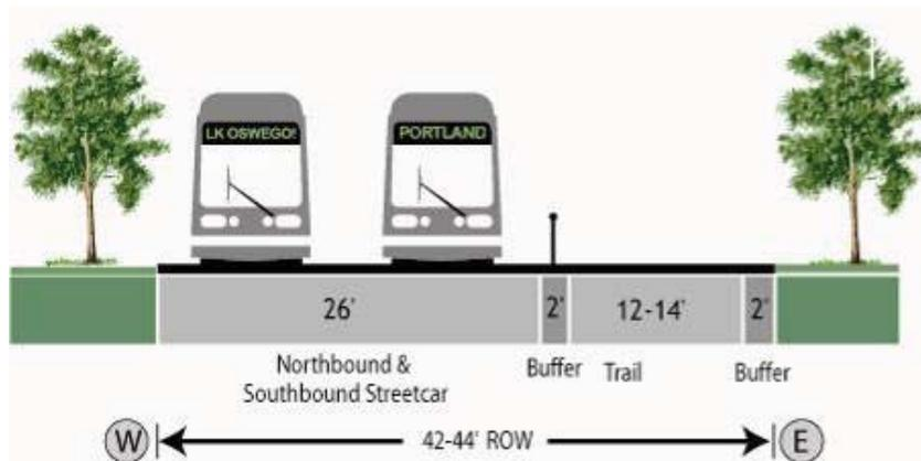
**Figure 4. Willamette Shore Line Alignment with Streetcar Design Option**
