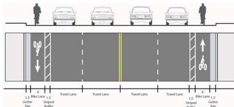
**Figure 18. Buffered Bike Lane Design Option**
