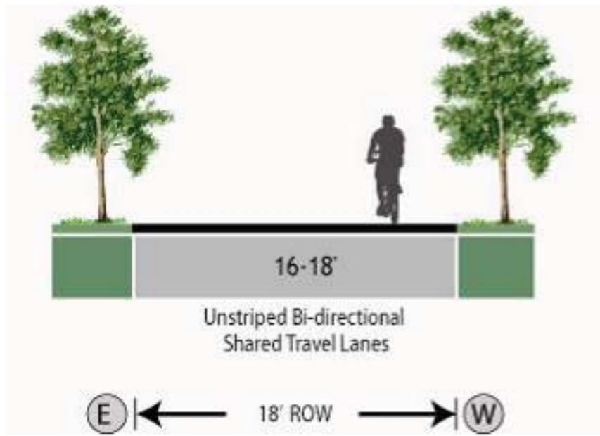
**Figure 63. Section 3.1a Bicycle Boulevard Improvements on Fielding**
