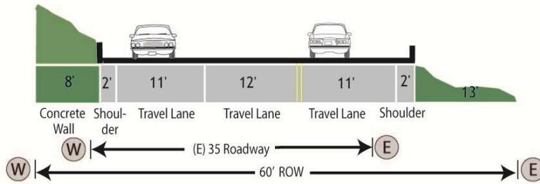
Shift Roadway West and Bench Cycle Track onto Roadway
