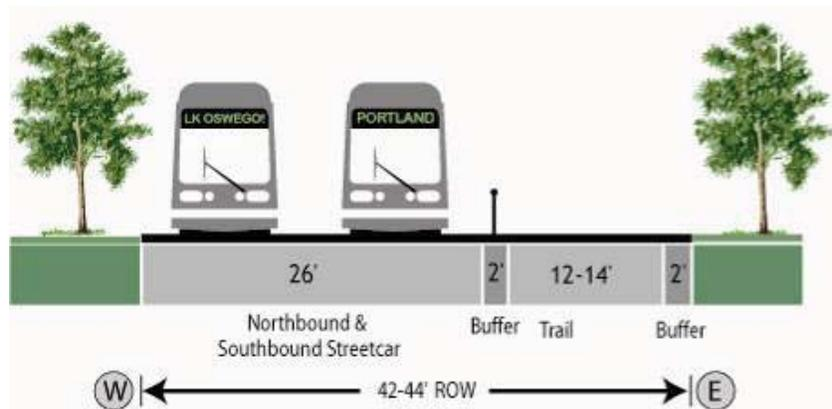
**Figure 22. Section 1.0a Willamette Shore Line with Double-track Streetcar**
