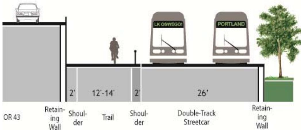
Figure 43. Section 2.1a Willamette Shore Line with Double Track Streetcar
