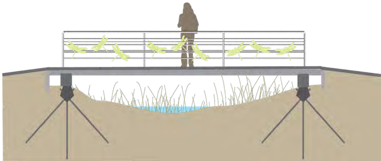
Figure 8 Steel and concrete structure showing anchoring and thematic elements
