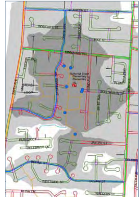
Map 3.4: Sidewalk gaps GIS analysis identified sidewalk gaps and school “walksheds.” The dark gray area above is within one quarter mile walking distance of access points to Butternut Creek Elementary School. Red lines indicate missing sidewalks.
