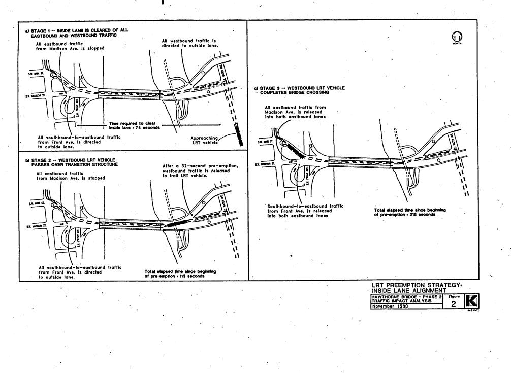
traffic must continue to be excluded from the inside lanes. Only after the LRT vehicle has passed completely over the bridge structure can opposite-direction traffic be released into the inside travel lane (see Part C). The total estimated preemption time required for opposite-direction traffic as shown in Parts A, B, and C of Figure 2 is 218 seconds or slightly over 3.5 minutes.
