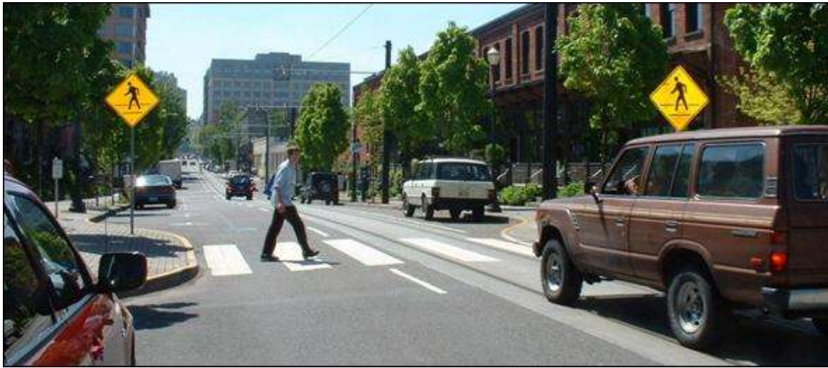
Curb bulb outs reduce the distance that people walking have to cover when crossing the street. Photo: Federal Highway Administration Pedestrian Safety Plan
