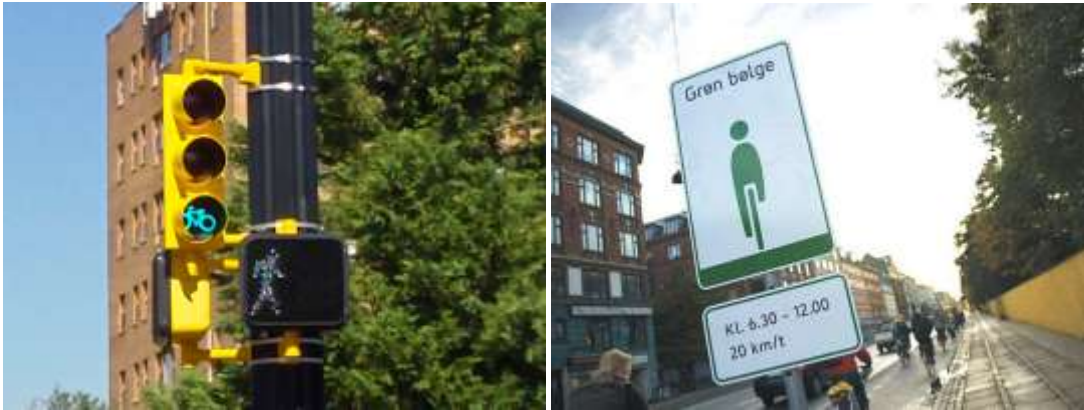
A bicycle signal in Portland. A sign in Copenhagen indicating that the bicycle route is a “green wave” route where traffic signal timing allows bicyclists to travel at a pace of approximately 12 miles per hour without stopping. This saves the cyclists energy and momentum and can make the roadway safer for all users. Photos: Portland, Streetsblog.org
