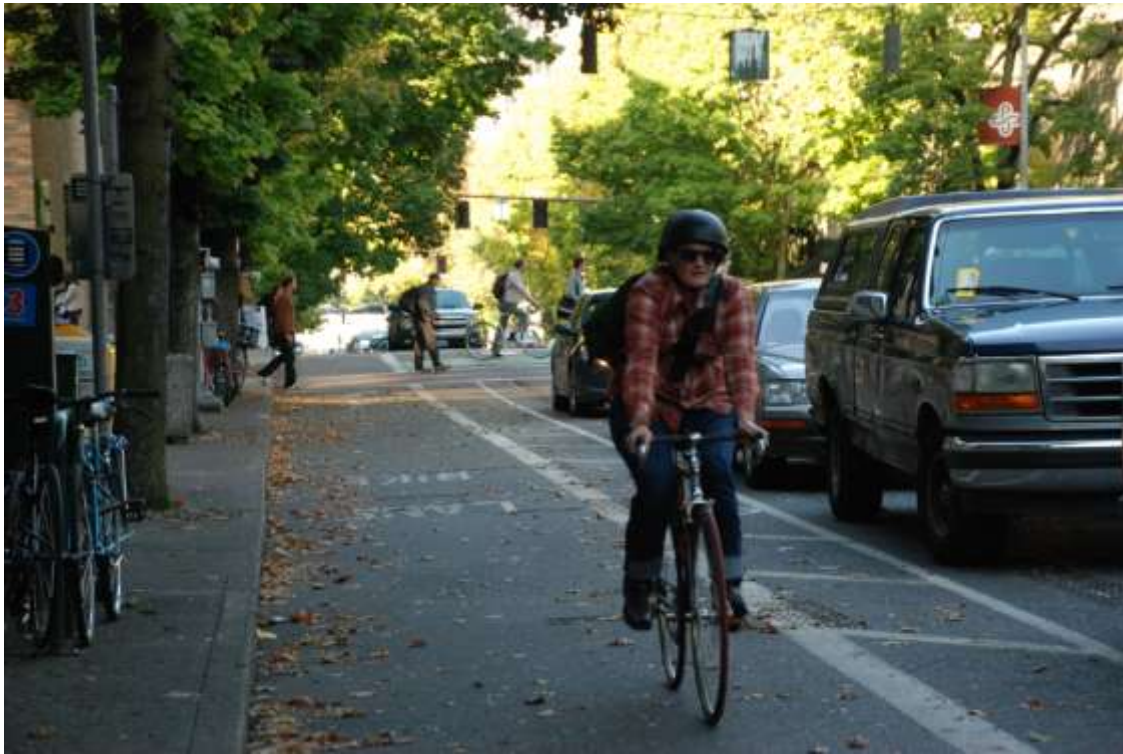
Moving the location of parked cars provides a cycle track near Portland State University. Photo: City of Portland
