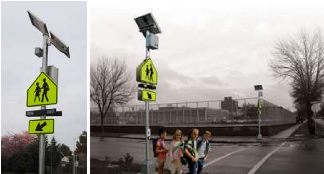
Elements such as rapid flashing beacons help prioritize pedestrian travel and improve safety. Photos: City of Tigard, Rapid Flashing Beacon
