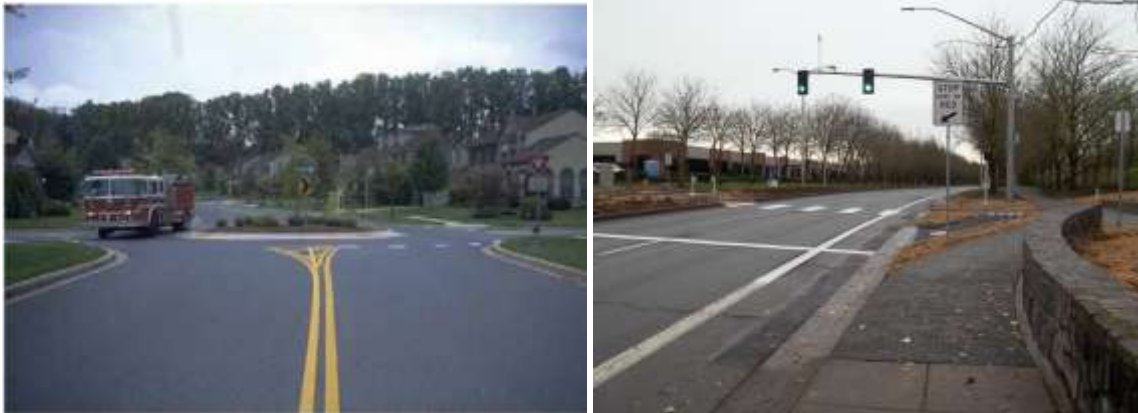
The photo on the left shows a roundabout that accommodates large vehicles and slows traffic in a residential neighborhood. The photo on the right shows a median on Evergreen in Hillsboro and a connection to the Rock Creek Trail. Photos: Federal Highway Administration, Washington County
