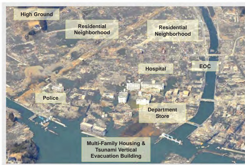
Critical Facilities in the Tsunami Zone – Minamisanriku, March 14, 2011. Because their hospital, emergency operation center, and other government and community service facilities were located in the tsunami inundation zone, the surviving community lost nearly all of its capacity to respond and implement recovery efforts. Source: Asia Air Survey Co., Ltd.
