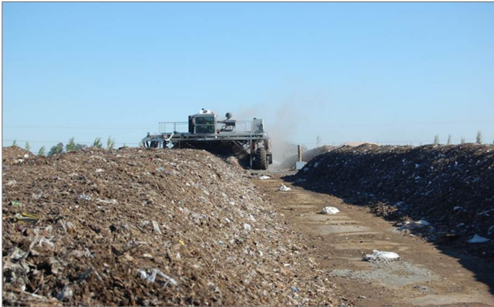
Figure 4 - Example of a Windrow Aerobic Composting Facility
