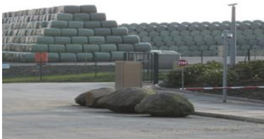
Figure 10 - Example of Stockpiled RDF
