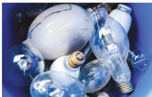
the mercury will be safely extracted, and the glass and metal end caps will be reused.
