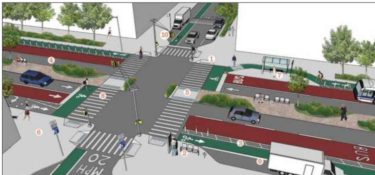
Example of a Vision Zero Street 22 (1)ADA Accessibility, (2)Public Amenities, (3) Protected Bike Lanes, (4) Narrow Vehicle Lanes, (5) Pedestrian Islands, (6) Wide Sidewalks, (7) Dedicated Mass Transit Facilities, (8) Signal Protected Pedestrian Crossings, (9) Dedicated Unloading Zone, (10) Signal Retiming
