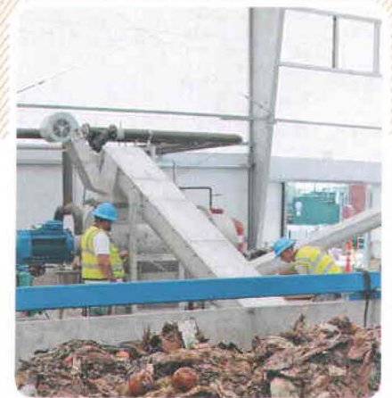
Food waste from post-consumer commercial sources is processed to remove contaminants such as metals and plastic as an initial step in producing biogas.
