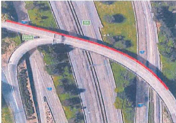
Bridge #08194, Hwy 3 over I-5, 372' Protective Fence Install protective fencing on the sidewalk side only.
