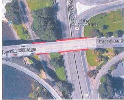
Bridge #06767A, US26 Ross Island Bridge over SE Grand Ave/SE McLoughlin Blvd, 227' Protective Fence
