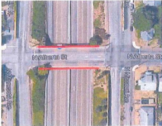
Bridge #09007, N Alberta St over I-5, 235' Protective Fence
