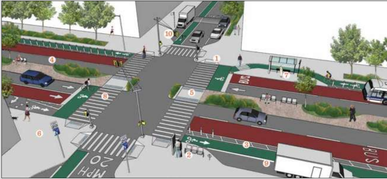
Figure 50: Example of a vision zero street (1)ADA accessibility, (2)public amenities, (3) protected bike lanes, (4) narrow vehicle lanes, (5) pedestrian islands, (6) wide sidewalks, (7) dedicated mass transit facilities, (8) signal protected pedestrian crossings, (9) dedicated unloading zone, (10) signal retiming Source: Vision Zero Streets.org
