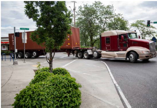
A truck apron in the St. Johns Town Center allows a large freight truck to make a turn while slowing other turning vehicles and providing additional buffer between traffic and pedestrians waiting to cross the street.
