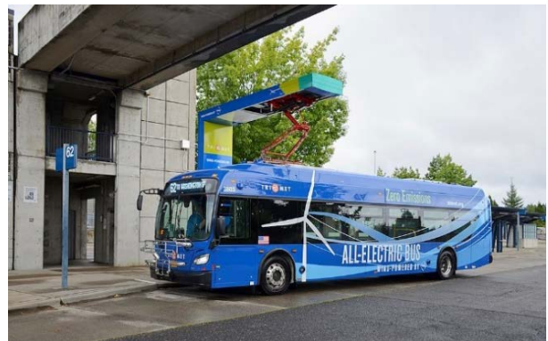
TriMet's new battery-electric bus charging at Sunset Transit Center, Photo courtesy of TriMet
