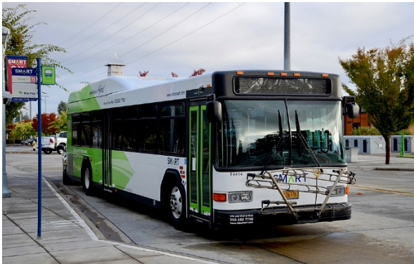
Low floor hybrid electric bus at Wilsonville Station, Photo courtesy of SMART
