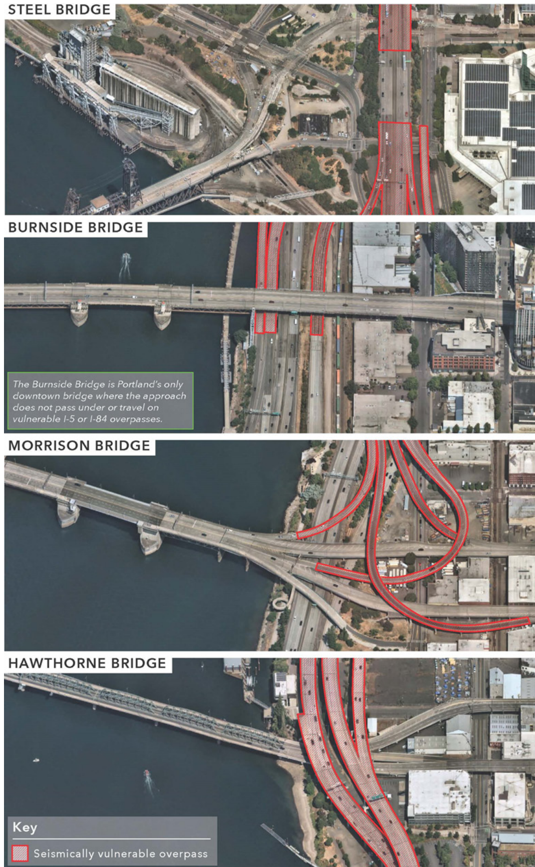
Figure 1.4-3. Seismic Vulnerability of Downtown Bridge Approaches
