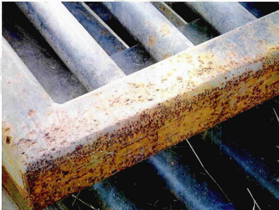
Photo A24: Tube Steel Gates – Typical Corrosion and Pitting
