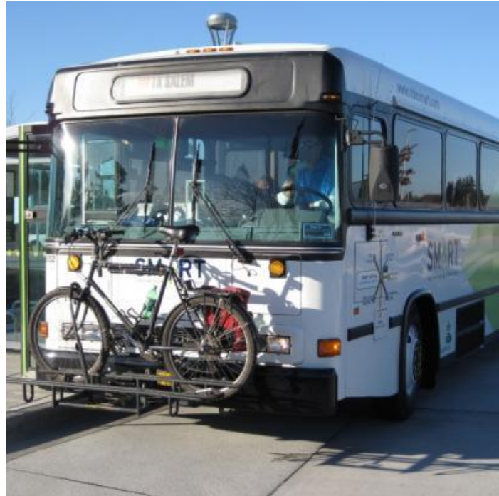
TriMet and SMART buses are equipped with bike racks that hold 3 bicycles Photo courtesy of SMART
