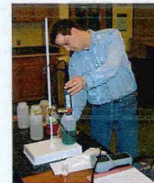
Calibrating the Water Quality Probe
