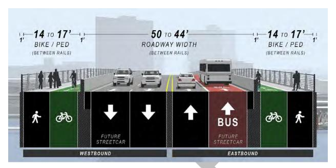
Figure 8.10 Earthquake Ready Burnside Bridge Proposed Typical Cross Section
