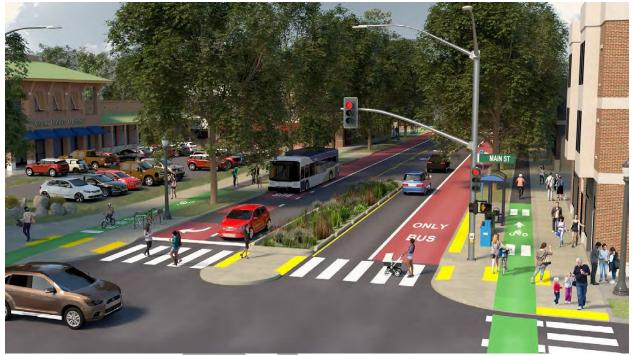
Rendering of a Regional Street showing a four-lane street with a planted median, crosswalks, and buildings. One lane in each direction is a bus only lane. There is a bus and four cars. A painted green bikeway and sidewalk are separated from the roadway by a planted median. People are walking and crossing the street. Source: Metro Designing Livable Streets and Trails Guide
