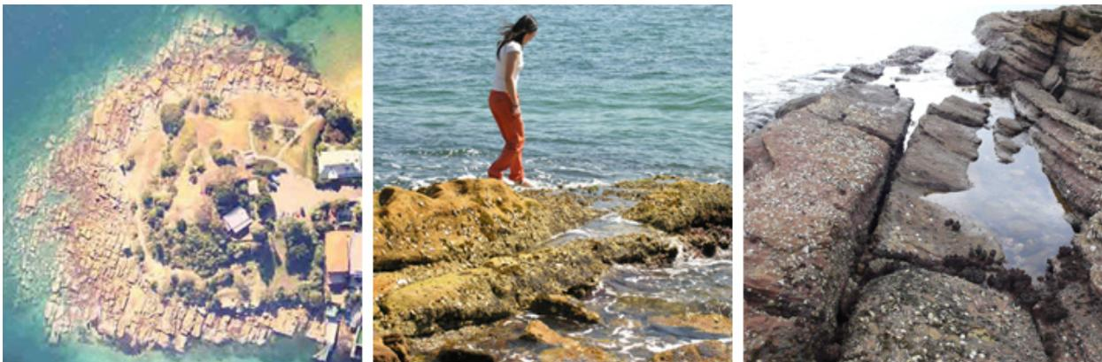
**Figure 3, Sandstone blocks were extracted from on-site, weathered using water jetting, and placed around the margins of Barangaroo Reserve.**
