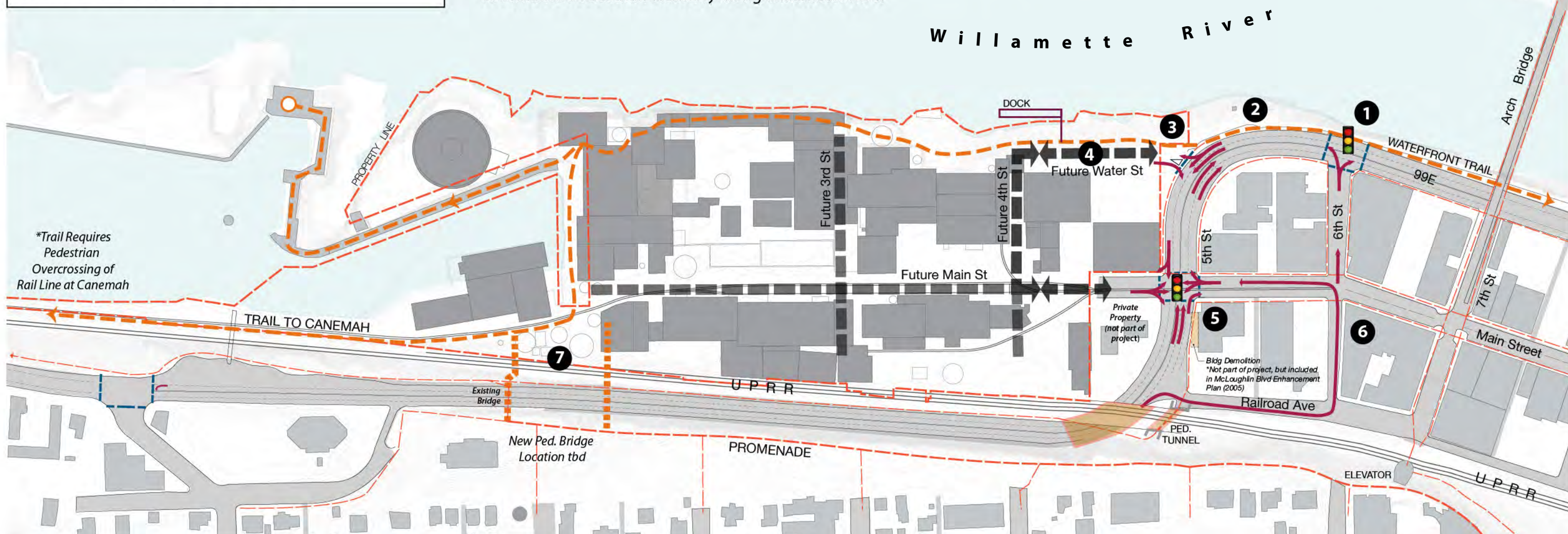
OPTION: Remove 1 NB Lane on McLoughlin, shift lanes to enhance Pedestrian Walkway along Willamette River
